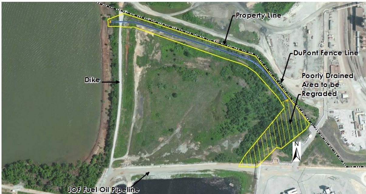
Figure 5. Phase 1 - North Drainage Culvert Limits
