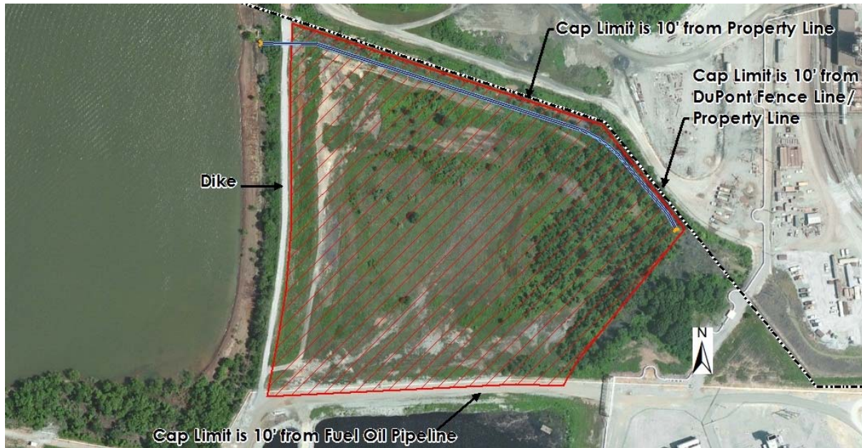
Figure 6. Phase 2 – Cap Installation Limits
